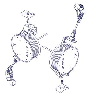
The extension cable swivels on a 360° axis. The swivel roller guide is to be adjusted to the cable extension direction and secured (screw connection) in this position.
