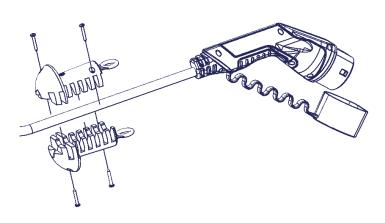
The length of the available cable can be individually adjusted with the provided cable stopper. The reliable clamping adapts to various cable diameters between 6 and 16 mm. For a thicker cable, a larger version is available. The stopper also serves as a safeguard against a full unload of the spring if the cable is unintentional released. It should therefore never be removed.
