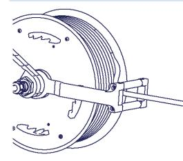
Fitted with four rollers, the roller guide ensures that the cable is correctly guided. It can be operated in a fixed or flexible mode. The roller guide adjusts then to the direction of the pull. The guide ensures that the cable is always guided onto the reel and prevents it from sliding of the drum.
