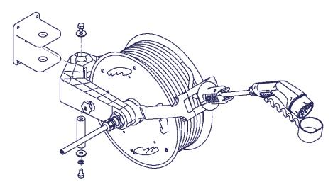
The cable reel can be rotated 150°.
