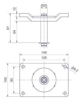
Mounting fixture WB 038 is included in the scope of supply, but no fastening screws.
